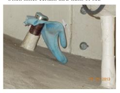
cocks are abandoned in place. They very much should be properly capped. If it is a seacock abandoned the lever should be in the closed position and the seacock should be capped. If the thru-hull fitting has only a sprue or stem, it can be capped by using a short piece of hose, clamped to the sprue or stem and a solid plug clamped in to open hose end. These should preferably be double clamped at both ends. As we can see in this photo, a rubber glove is not the answer. Don't do that !!
