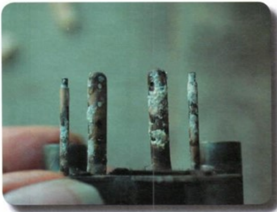
Older aluminum carburetors tend to suffer from the corrosive effects of ethanol much more than newer ones, which are made out of more resistant alloys. Corrosion can block tiny orifices, causing hard starting and rough running.
